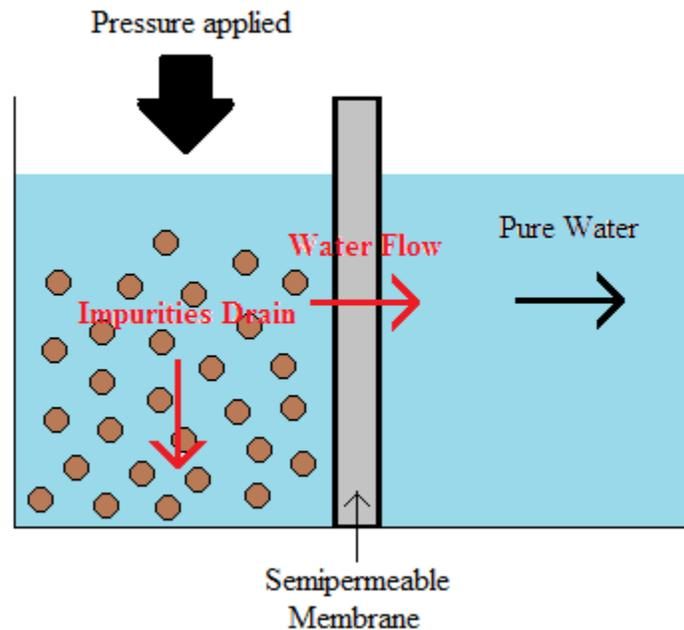
Membrane filtration uses very fine filter membranes of varying pore size to filter out fine particulate matter, [pathogens](#) and, depending on the pore size of the filter, ions. With decreasing pore size, the amount of applied pressure required to force water through the membrane must increase, increasing energy costs (Witgens, 2005).
